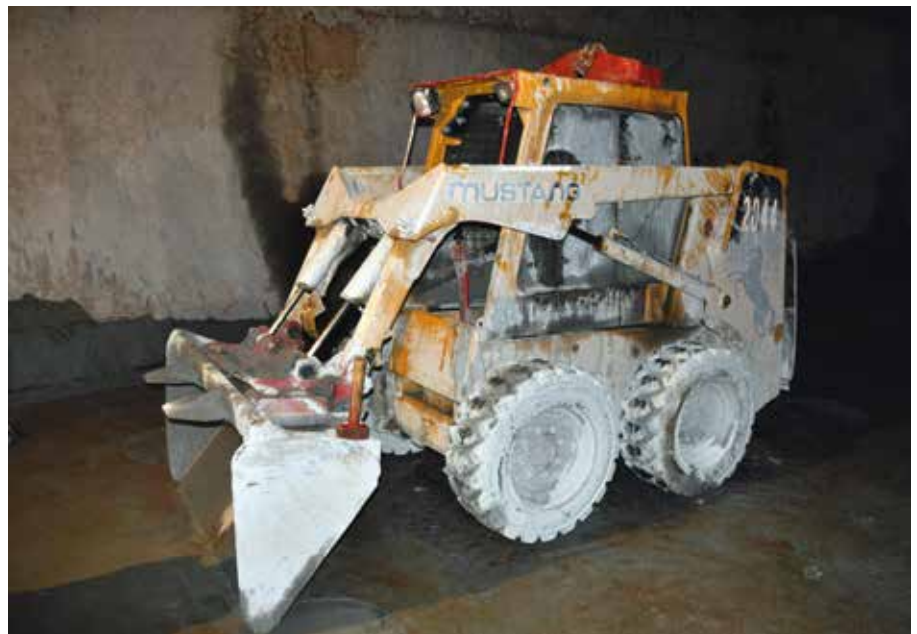
THE SKID-STEER LOADER: The able seaman was repairing this skid-steer loader when he got crushed between the bucket and the operator's compartment. Today there are no clear regulations for the use of such loaders on board a vessel. The Norwegian Maritime Authority has now been requested to draw up relevant regulations.
