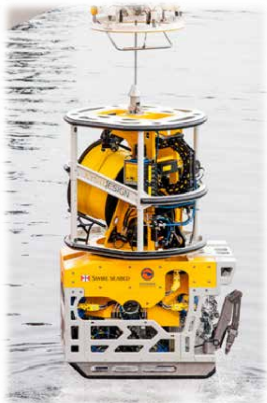
Kystdesign Supporter WROV med tether management system (TMS)
